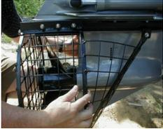
6. Once the front screen is secured to the guard, tighten the last two 1/4-20 bolts at the front of the harness.
