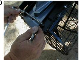
**Note:** If your harness has a 5/16" full threaded bolt, the two flange nuts should be installed on the bolt between the legs of the harness at this point. They will be secured during Step #8.
