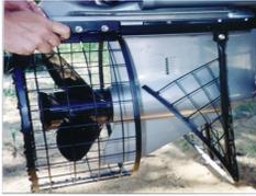
5. Pull the front screen rearward to the outer rim of the guard. The rim of the front screen fits over the guard rim. Using the 1/4-20 x 3/4" long bolts and locknuts, secure the front screen to the guard. You may use the enclosed cable ties instead of the bolts. Starting at the "six o'clock" position, install the fasteners evenly upward finishing at the upper ends of the front screen. Two 7/16" wrenches are needed for this step.
