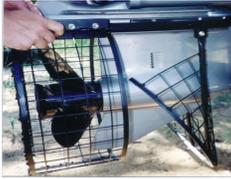
5. Pull the front screen rearward to the outer rim of the guard. The rim of the front screen fits over the guard rim. Using the 1/4-20 x 3/4" long bolts and locknuts, secure the front screen to the guard. You may use the enclosed cable ties instead of the bolts.
