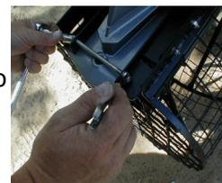
**Note:** If your harness has a 5/16" full threaded bolt, the two flange nuts should be installed on the bolt between the legs of the harness at this point. They will be secured during Step #8.
